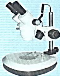
"GIPPON-JAPAN" GD-2P Stereo Microscope with co-axial focussing system and dual objectives (without illuminators)
